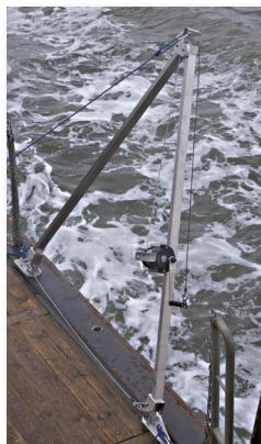
Mounting bracket Stainless steel, rust-free
